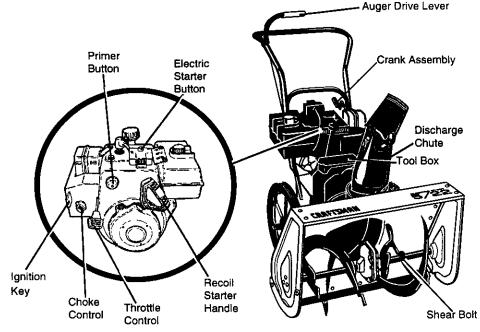
Auger Drive Lever – Starts and stops the auger and impeller (snow gathering and throwing). The auger assists in the self propelling.
